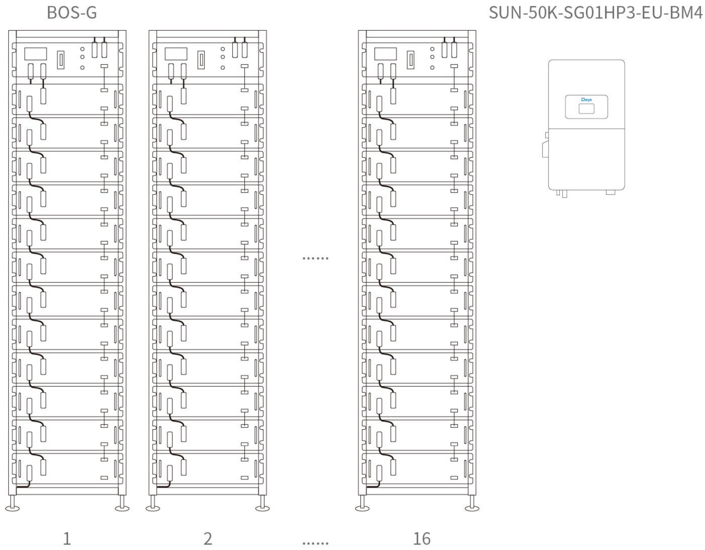
Maximum support for 16 racks of batteries in parallel
